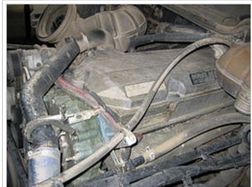
14 Litre S-60 view in a Freightliner Century S/T prime mover
